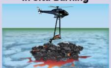
Vessels maneuver containment boom to contain and thicken the slick. Oil is then burned off the water's surface in a controlled fashion. Oil contained by ice may be able to be burned as well.
