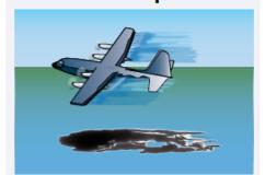
Chemicals are applied to the oil spill that break the slick into smaller droplets that mix into the water, avoiding contamination of areas like beaches or tide flats.
