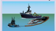
Vessels maneuver containment boom to capture and concentrate spilled oil. Oil is then removed from the water's surface with a skimmer. Recovered oil is stored and disposed of.
