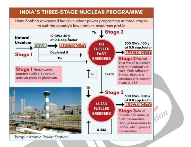
**Note:** The operationalisation of the **prototype fast breeder reactor (PFBR)** will mark the start of **stage II** of India's three-stage nuclear power programme.
