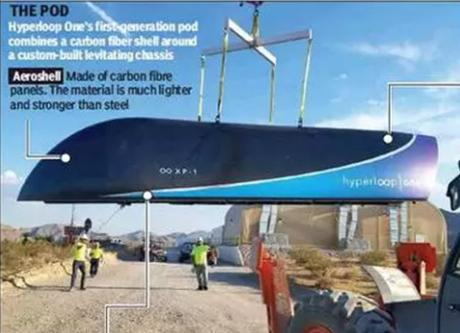
**Levitating chassis** is made of aluminium and houses the propulsion system and magnets for levitation and guidance. Its design is similar to a Formula 1 car. It is built like a shell to be lightweight but strong
